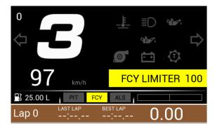
If the car speed is higher than the target limiter speed, check the tyre circumference selected on the ECU clx file (2100 mm as default) that should match with the size of the tires used on the car.
