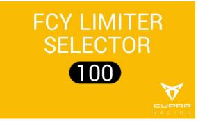
At the Race page, a new flag will be shown, where the driver can see when the limiter is active and the target speed limiter that is selected. With this layout, the driver can quickly check if the car speed is higher than the selected one.
